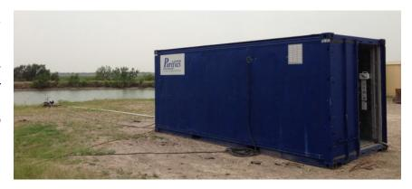
There is no pretreatment prior to the *Cuf* which eliminates the need for a clarifier and other pretreatment infrastructure. A small dosage of coagulant is added in-line where ultra coagulation occurs in the *Cuf* system. Coagulant dosage is less than the existing plant. No polymer or other process chemicals are added. The results of this pilot are consistent with other *Cuf* surface water pilot results.
